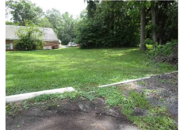
A rain garden can be installed in the turfgrass area south of the driveway to capture runoff from the pavement and allow it to infiltrate. The bioretention system will also provide a habitat for the local wildlife. A preliminary soil assessment suggests that the soils have suitable drainage characteristics for green infrastructure.
