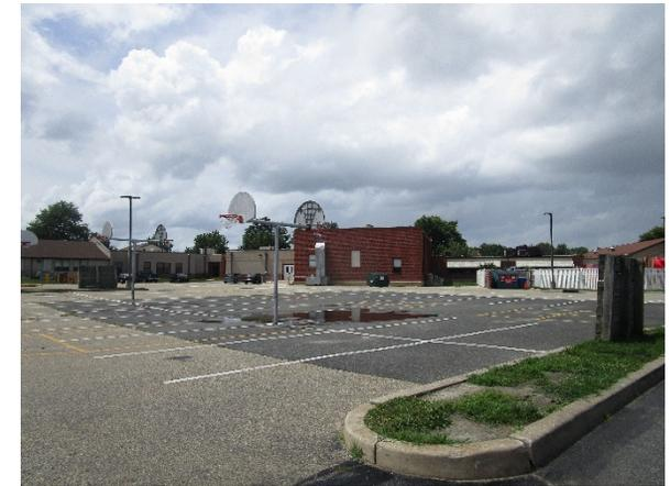
Rain gardens can be installed alongside the school at the northwest corner, northeast corner, and southwest corner of the building to capture stormwater runoff from the roof. A portion of the western parking lot can be replaced with pervious pavement to allow stormwater to infiltrate into the ground. A preliminary soil assessment suggests that more soil testing would be required before determining the soil's suitability for green infrastructure.
